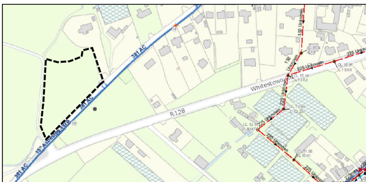
Figure 10.0 Extract from Irish Water Web Maps showing the existing foul network for Rush in red and the water mains in blue. The subject site is outlined in black. Note that an extension of the wastewater network is required to service these lands.
