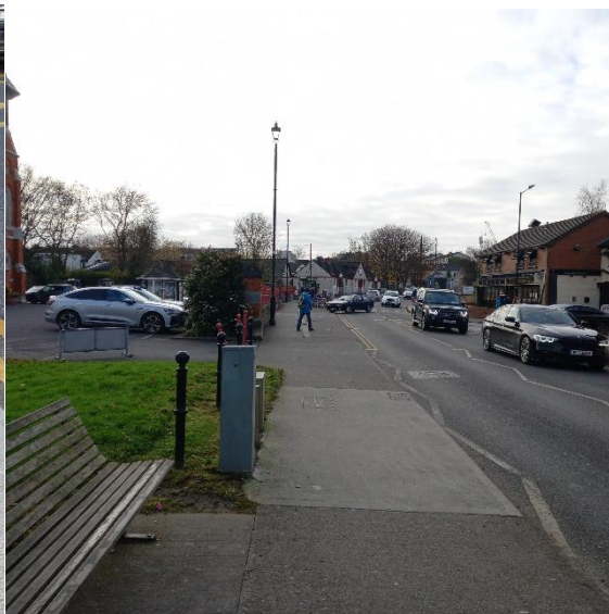
Desire lines, large radii junctions with undefined pedestrian routes close to Town Center Facilities and the lack of pavement contrast leave pedestrians, the visually impaired and mobility impaired isolated at primary crossing places.
