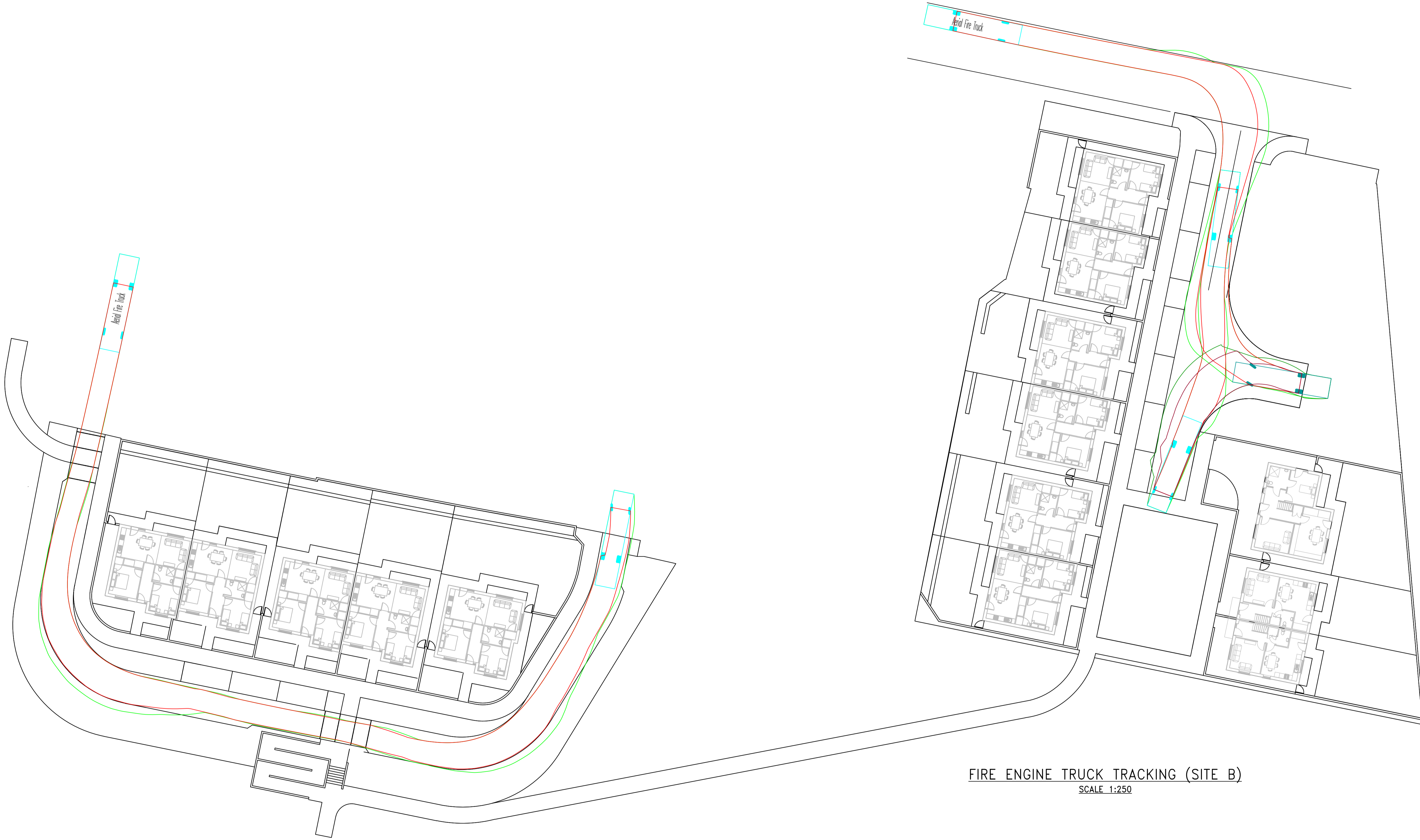
FIRE ENGINE TRUCK TRACKING (SITE A) SCALE 1:250
