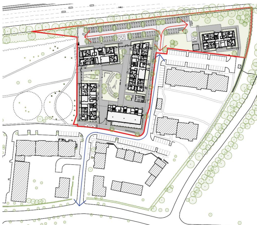
Site vehicular access and movement diagram – existing roads (blue) and new roads (red)
