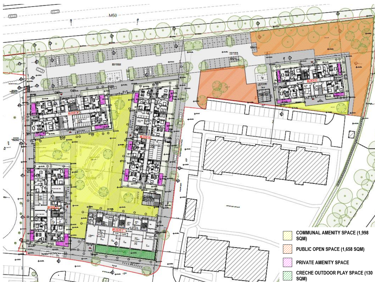
Diagram indicating open spaces - POS (orange), CAS (yellow), creche play (green), private amenity space (purple)
