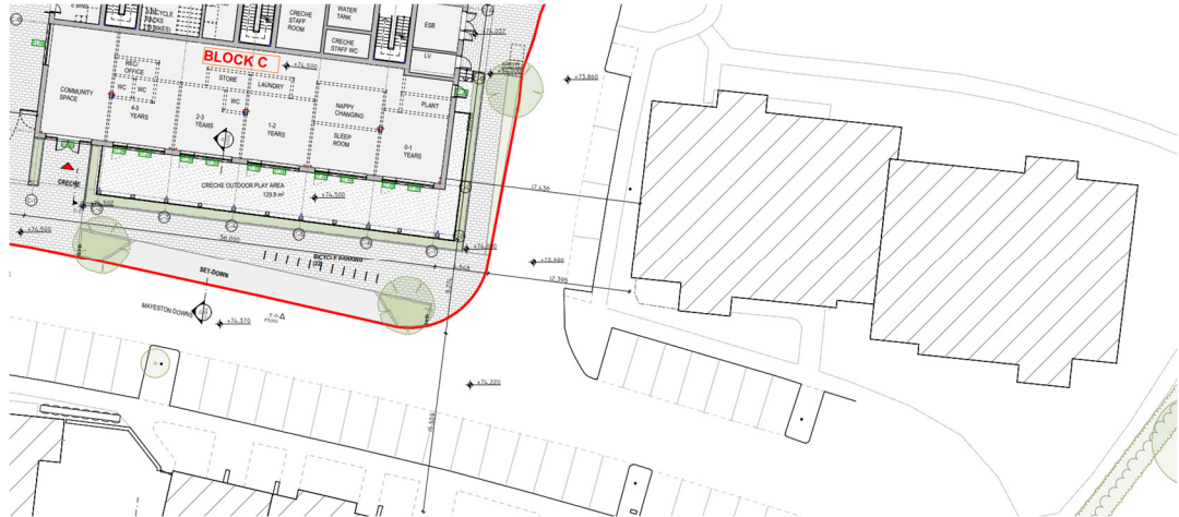
Figure 2.1 Visibility splays at junction
