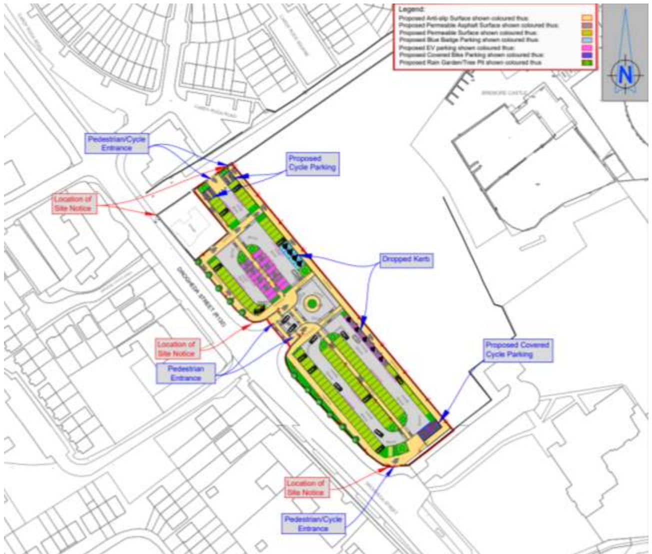
Figure 3 Bremore carpark showing proposed upgrade works
