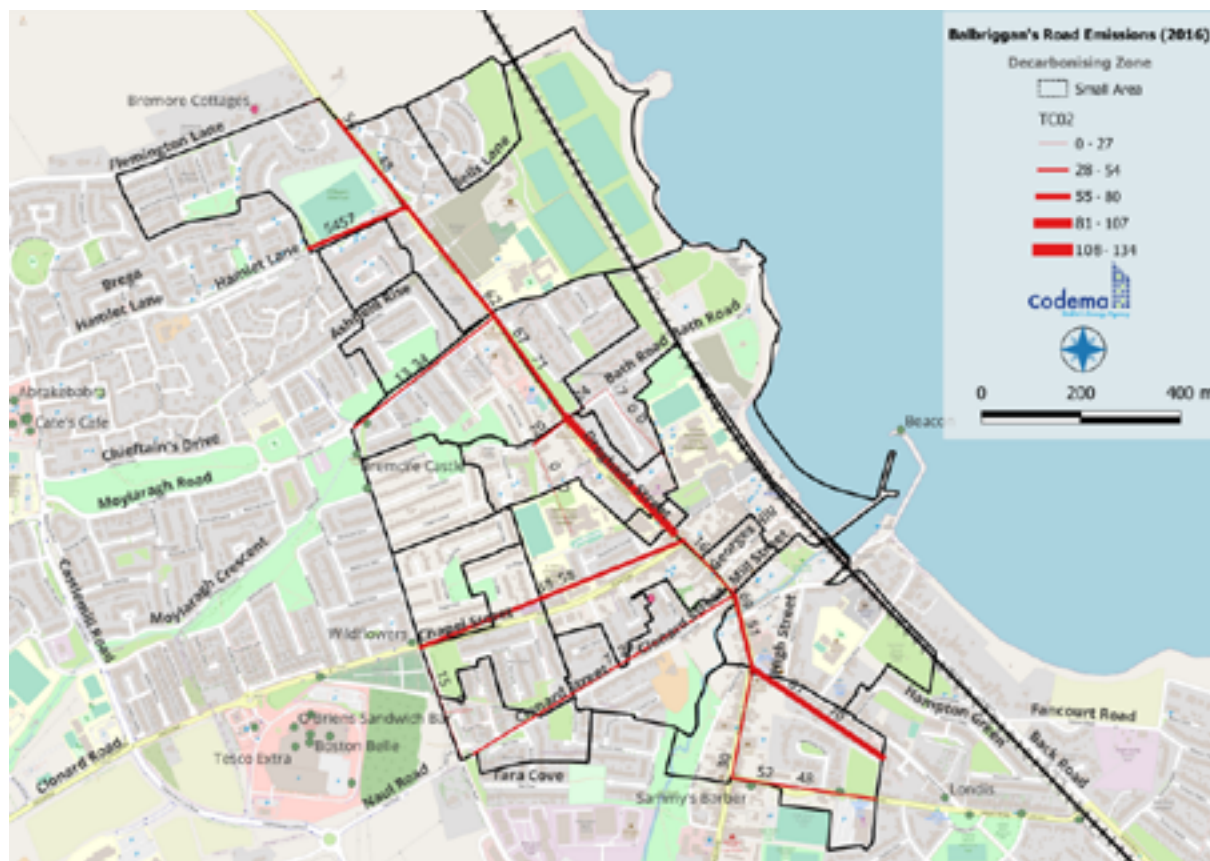
Figure 6.8: Road Emissions (tCO 2 ) – developed based on modelling data supplied by the National Transport Authority
