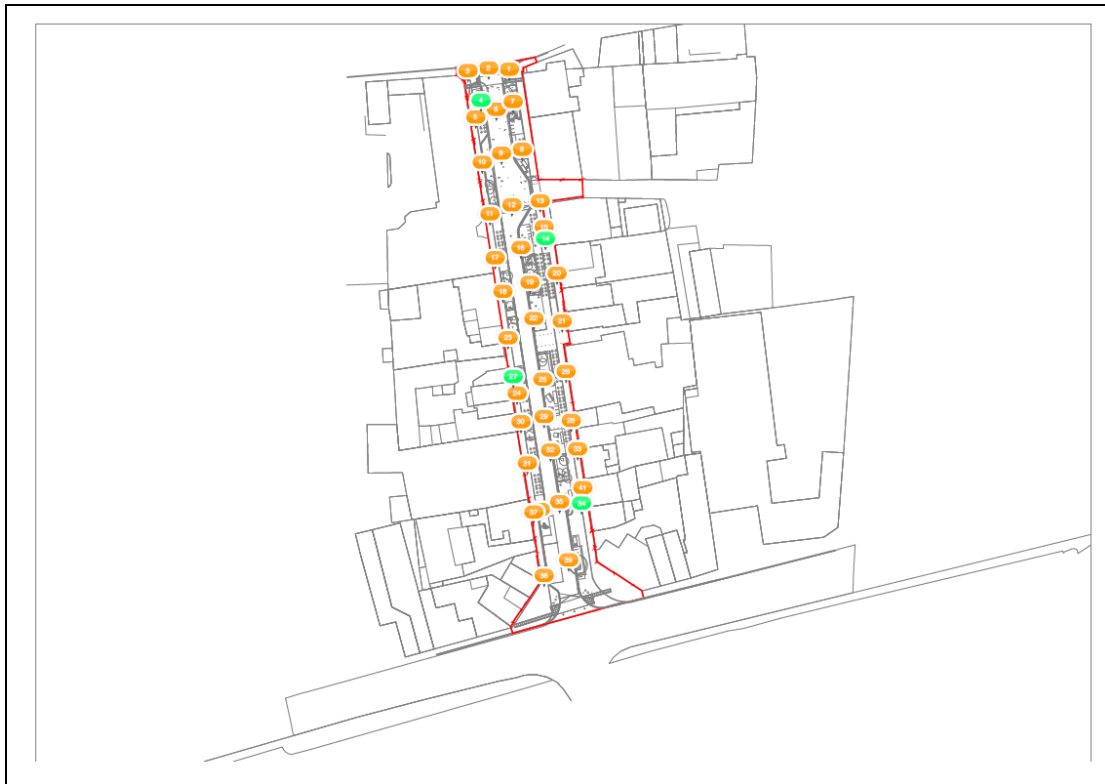
Figure 3.11. Existing light levels on New Street vary from 6.5 lux to 61.6 lux, giving an overall average of approx. 17 lux in the streetscape.
