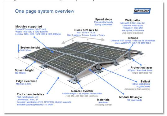
Below is a diagram to illustrate details of typical PV panel arrays.
