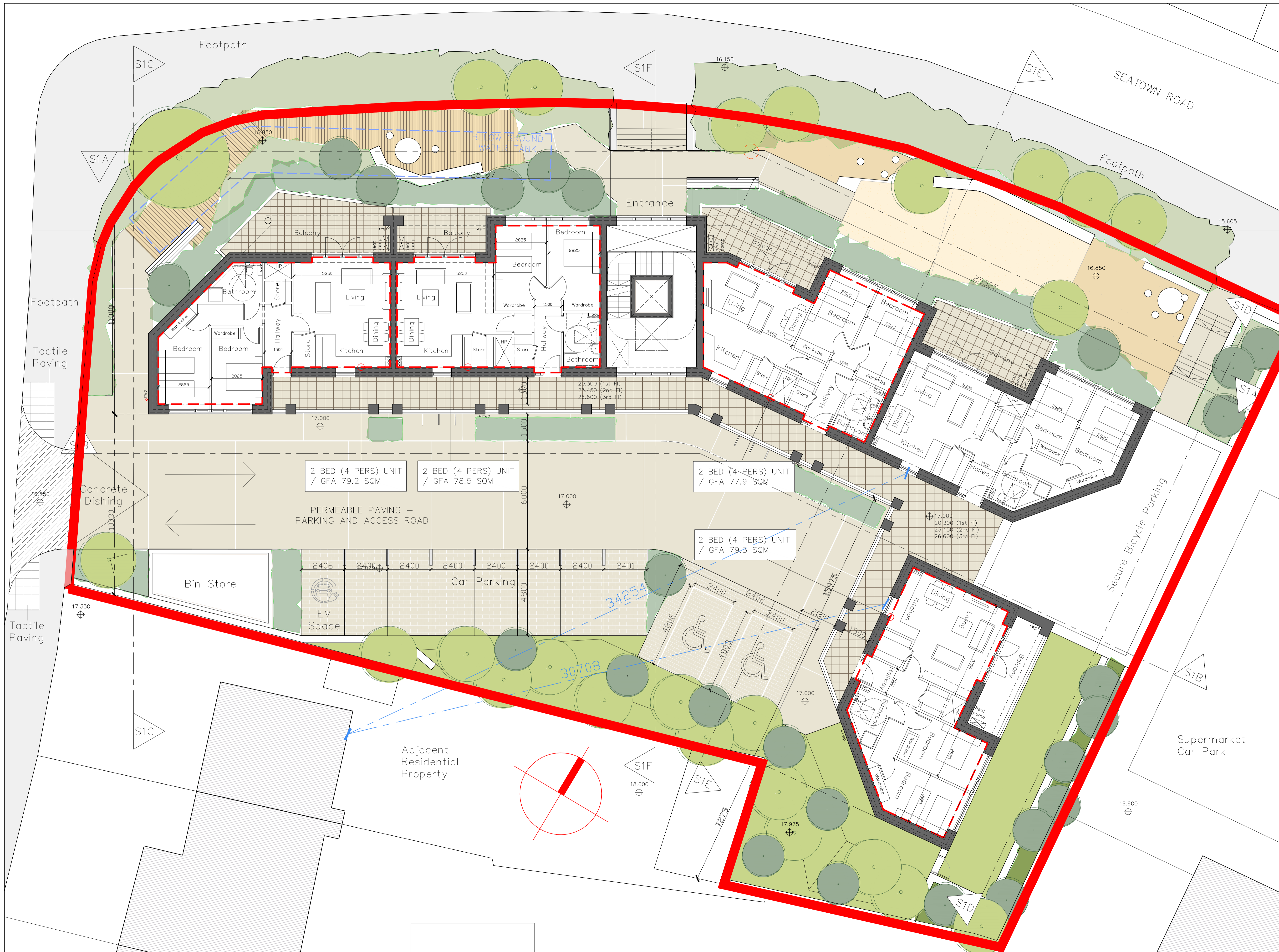
SITE NO 1 - PROPOSED FIRST / SECOND / THIRD FLOOR PLANS (SCALE 1:100)
