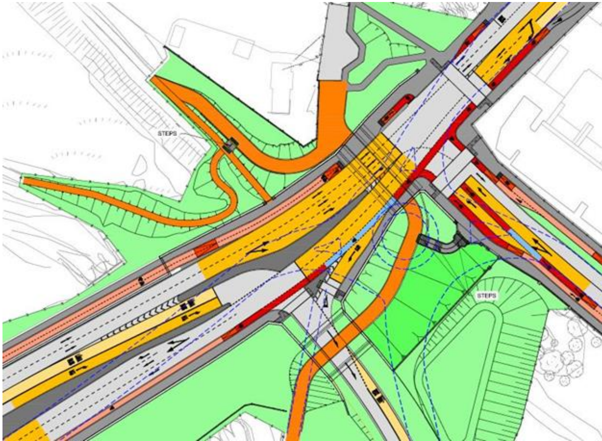
Figure 4 Schematic Detailing Lack of Direct Access to N3 Cycling Underpass, No segregated cycle lane to National Sports Campus.
