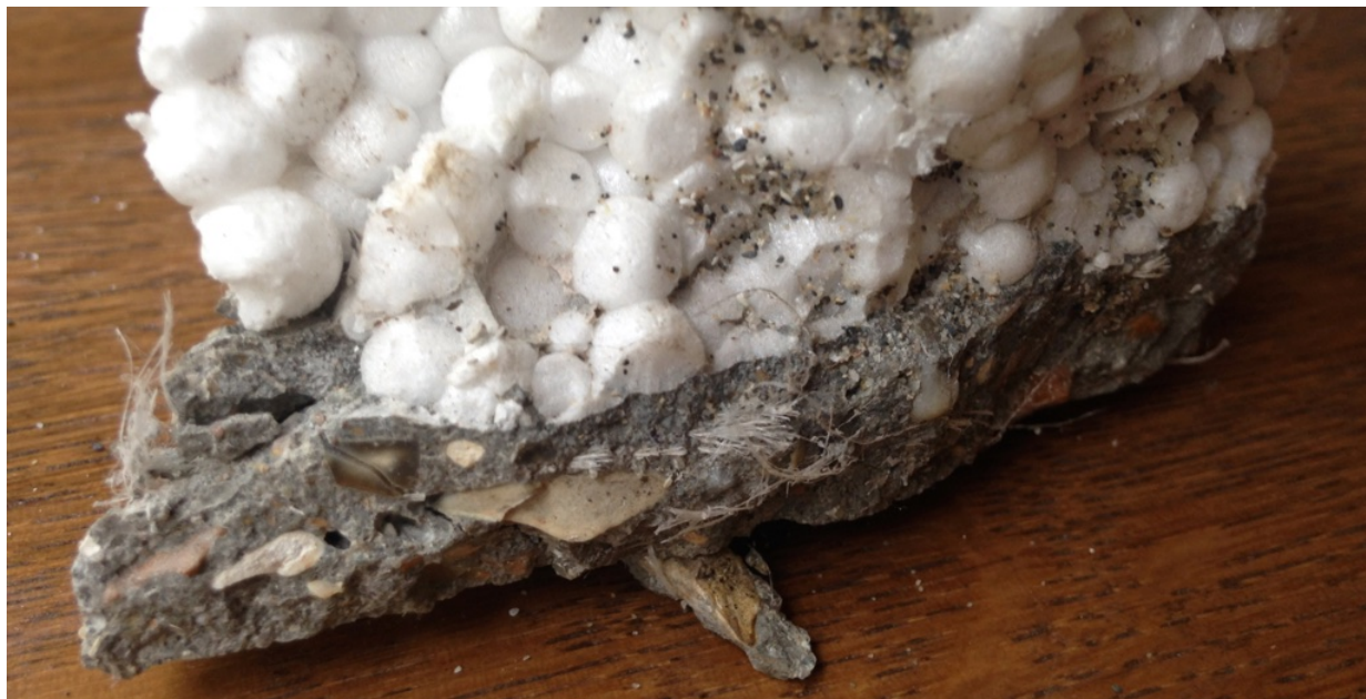
Figure 11: Illustrates the plastic shard composite material make-up of the cement used in the pontoon.
