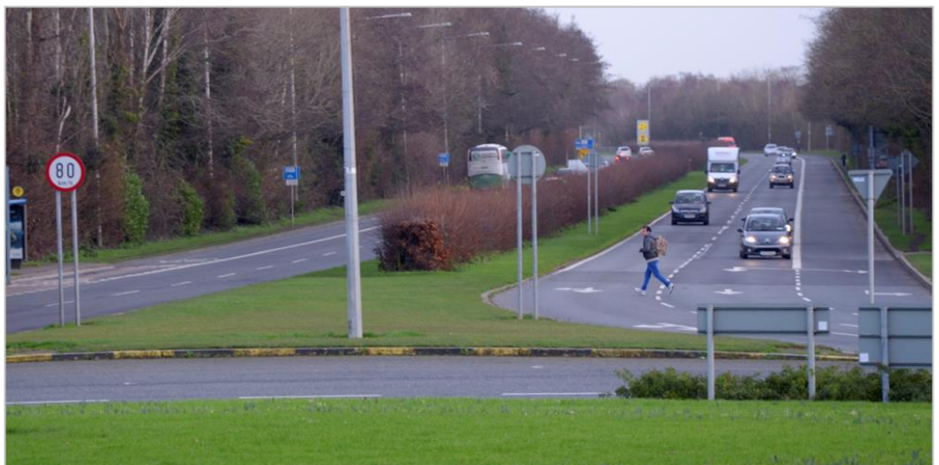
Figure 3.4: Lack of Safe Pedestrian Links to Bus Stops
