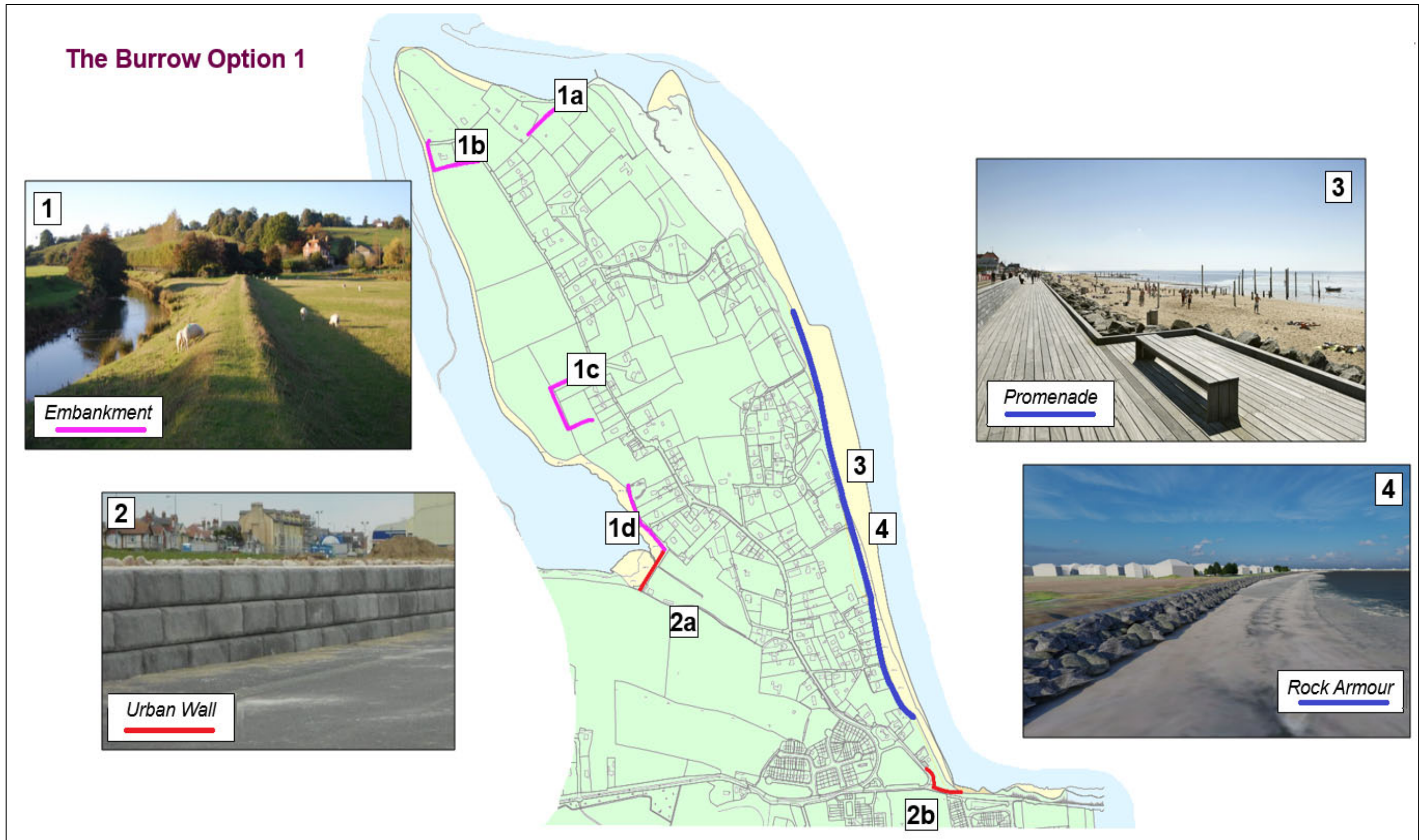
Figure 5.1: The Burrow Option 1 – Rock armour & Flood defences Plan View
