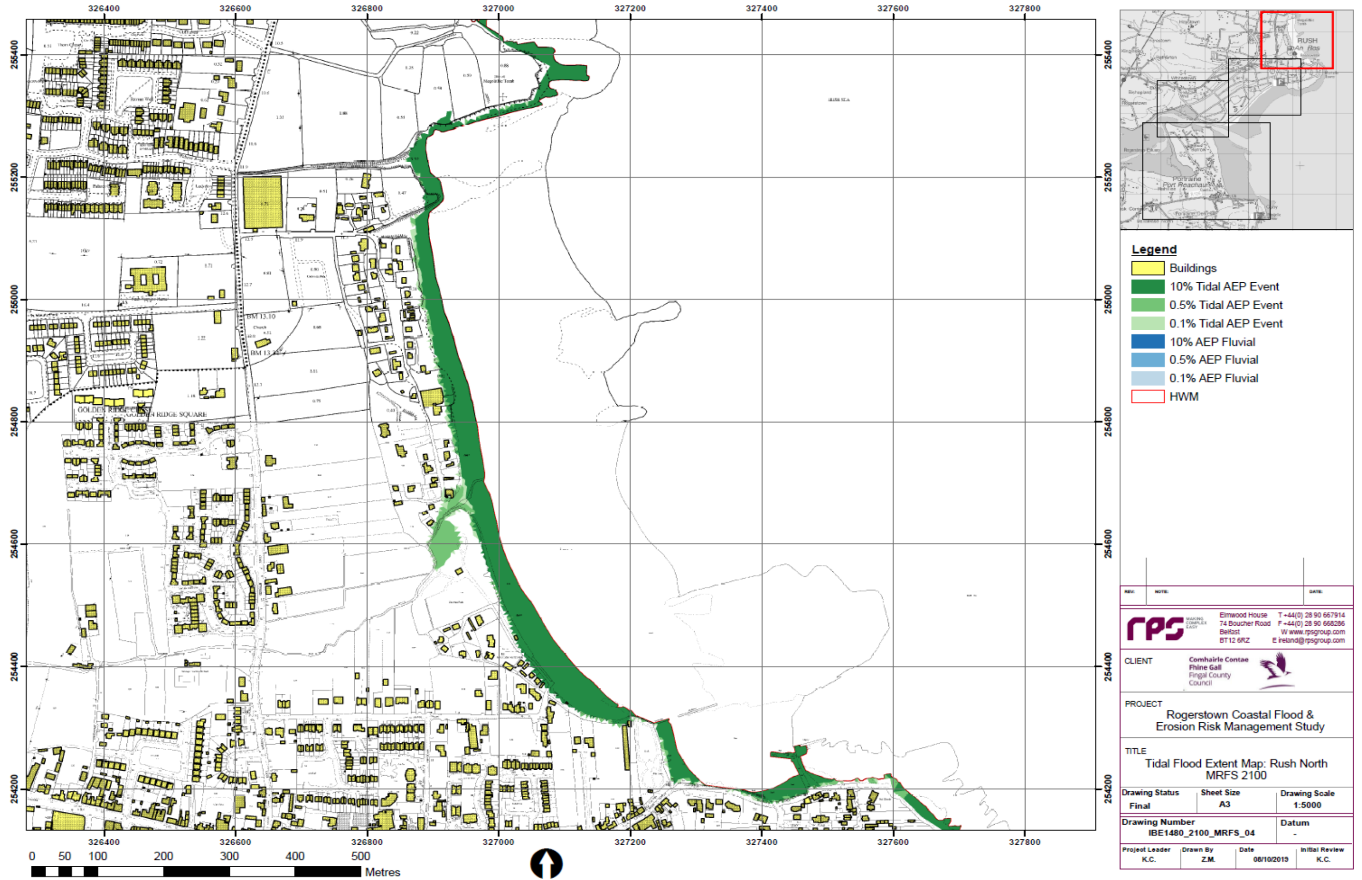
Figure 5.9: Tidal Flood Extent Map: Rush North - 2100 Medium Range Future Scenario (i.e. +0.50m sea level rise and c.4m of coastal retreat)
