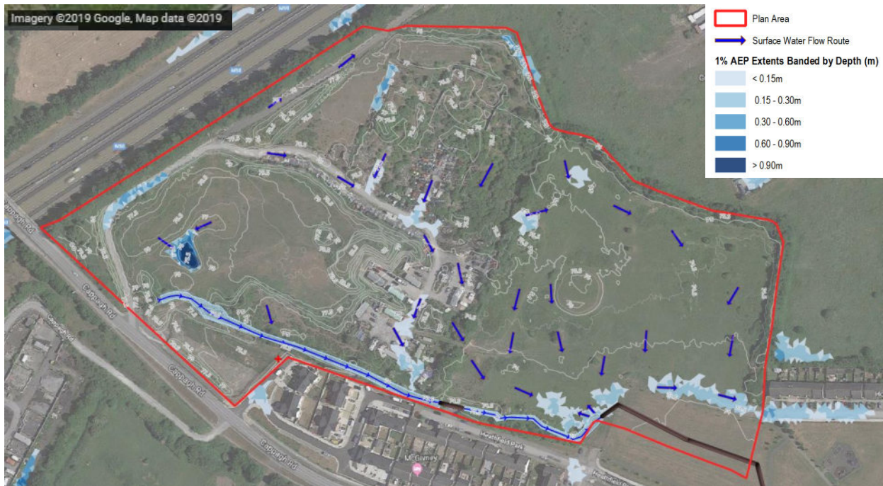
Figure 6.11 1% AEP Event Flood Routing
