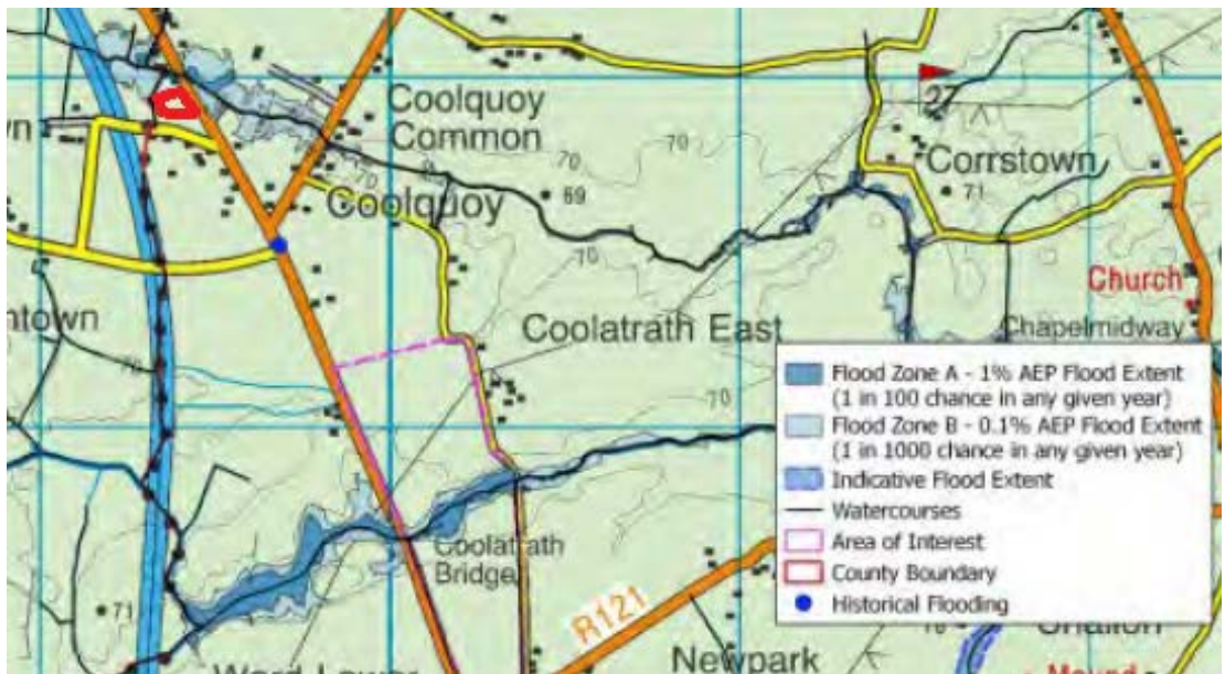
Figure 2 – Proposed development site and flood extents from unnamed watercourse as shown in the Strategic Flood Risk Assessment document within Fingal Development Plan 2017-2023.
