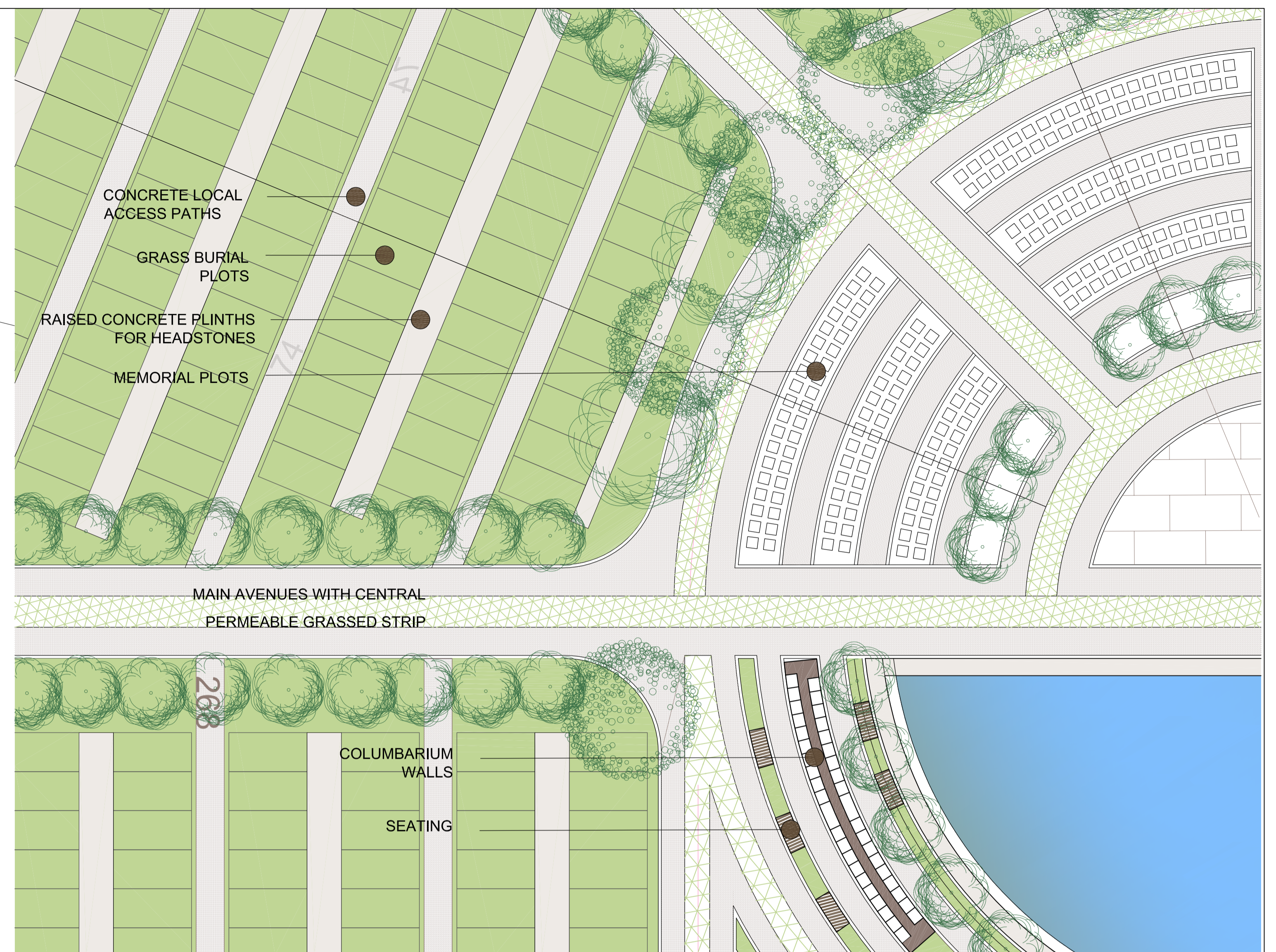
Detail of typical site arrangement scale 1:100
