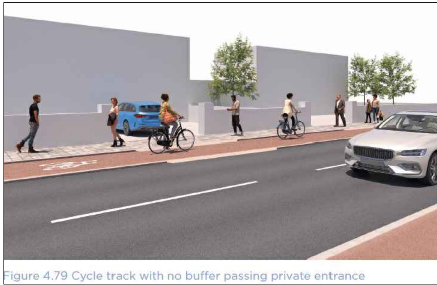
Figure 4.79 Cycle track with no buffer passing private entrance
