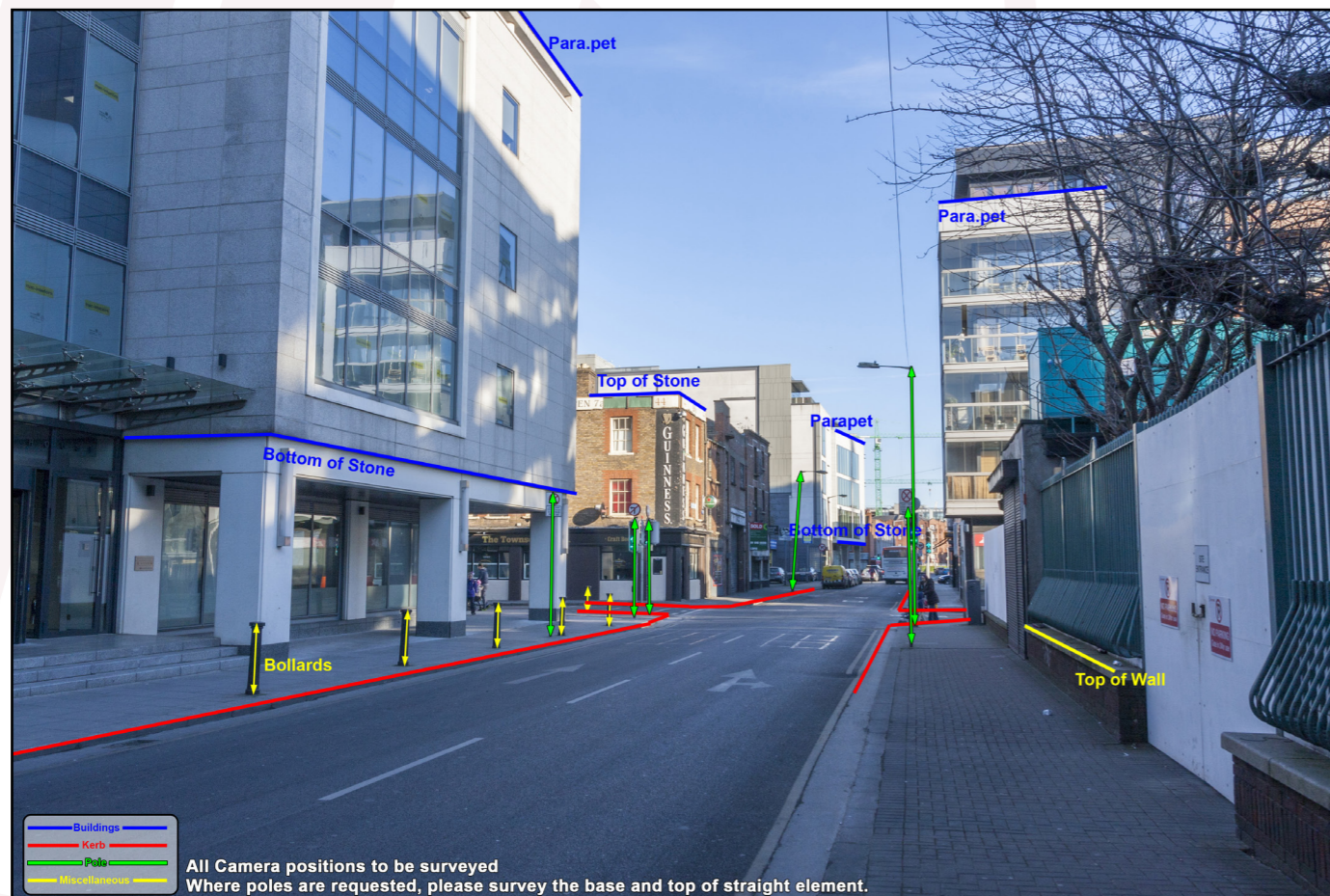
Fig.7: Fixed reference points marked for surveyour.
