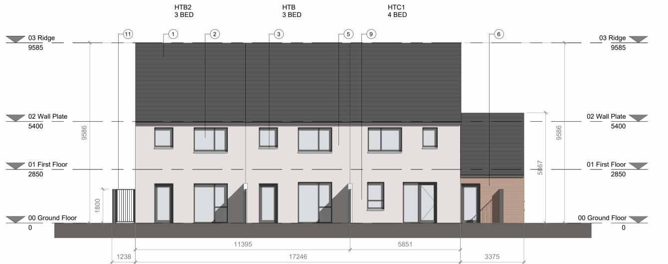
**Block Type A - Typical Rear Elevation**
