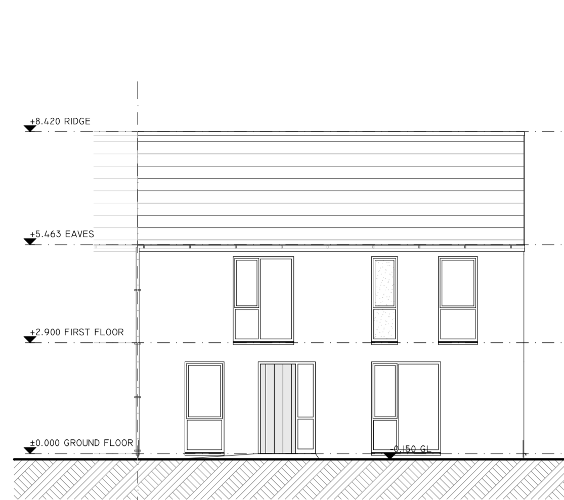
11 FRONT ELEVATION 1:100 TYPE F - END TERRACE, RIGHT GABLE WITH OPE.
