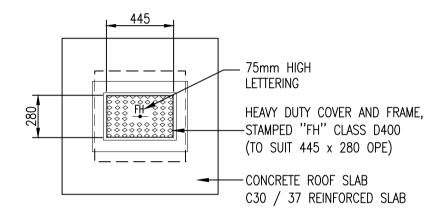
ON-LINE FIRE HYDRANT CHAMBER **ROOF PLAN**
