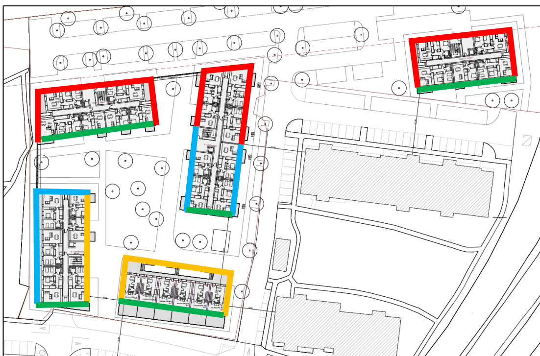
Figure 9 Mark-up of facades that require a minimum sound insulation specification on building elements.
