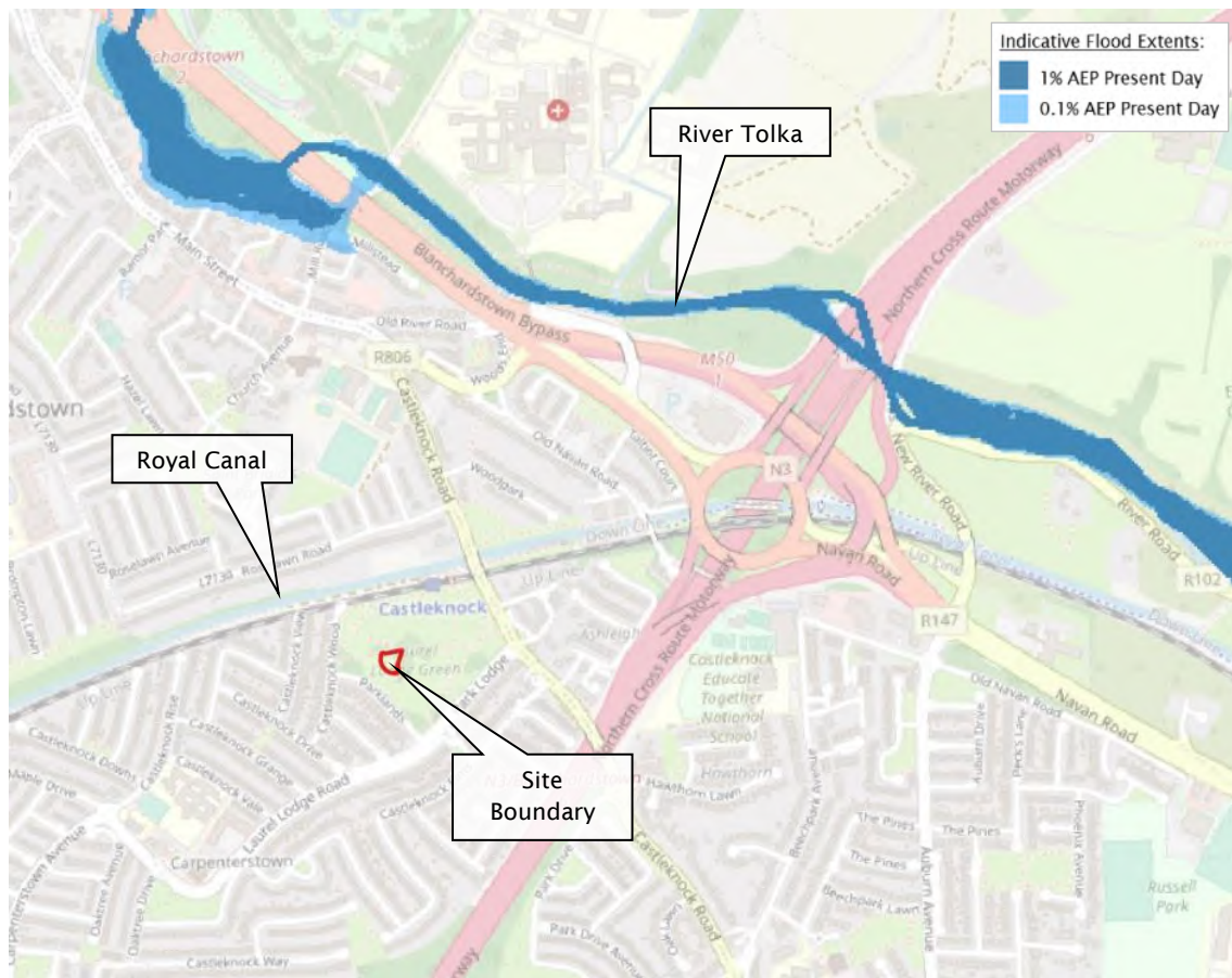
Figure 3.1: Extract from OPW NIFM Fluvial Flood Mapping
