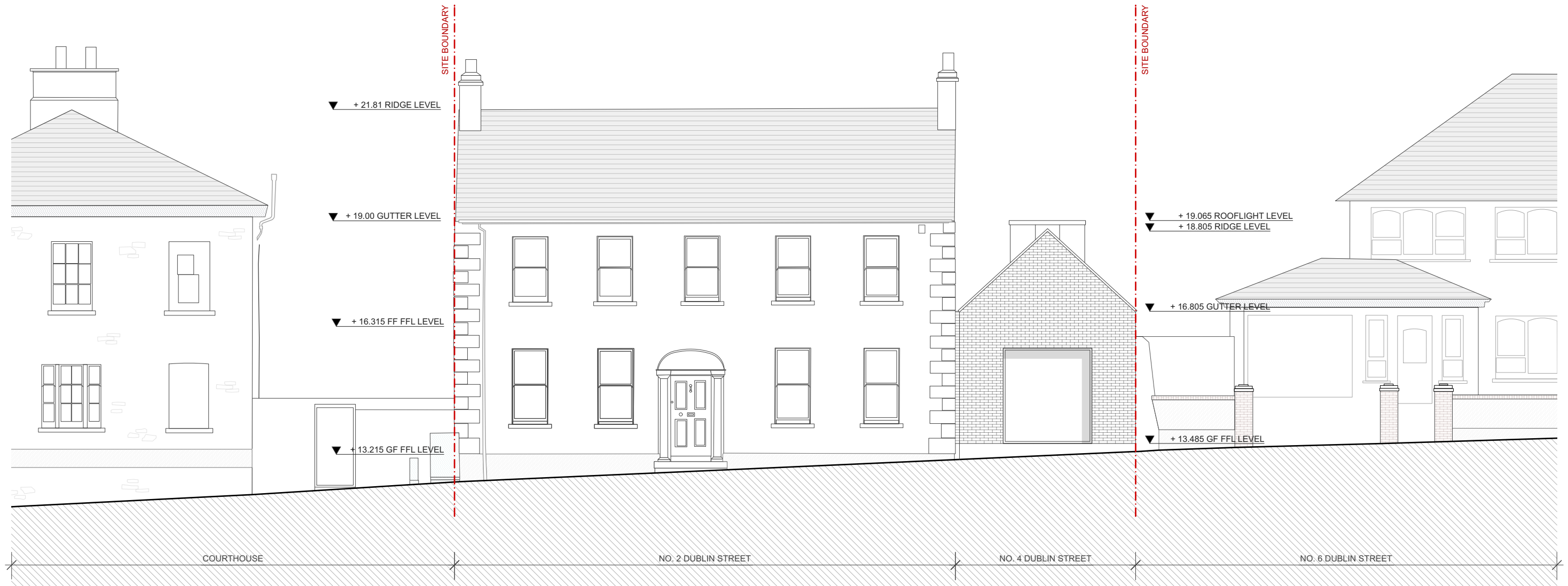
1 WEST ELEVATION - NO. 2 - 4 DUBLIN STREET PA-010 1:100 (A3)
