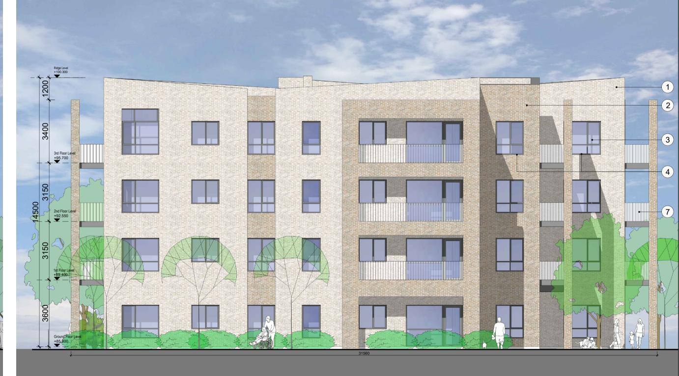
Apartment Block D - Proposed East Elevation Scale 1:100 @ A1
