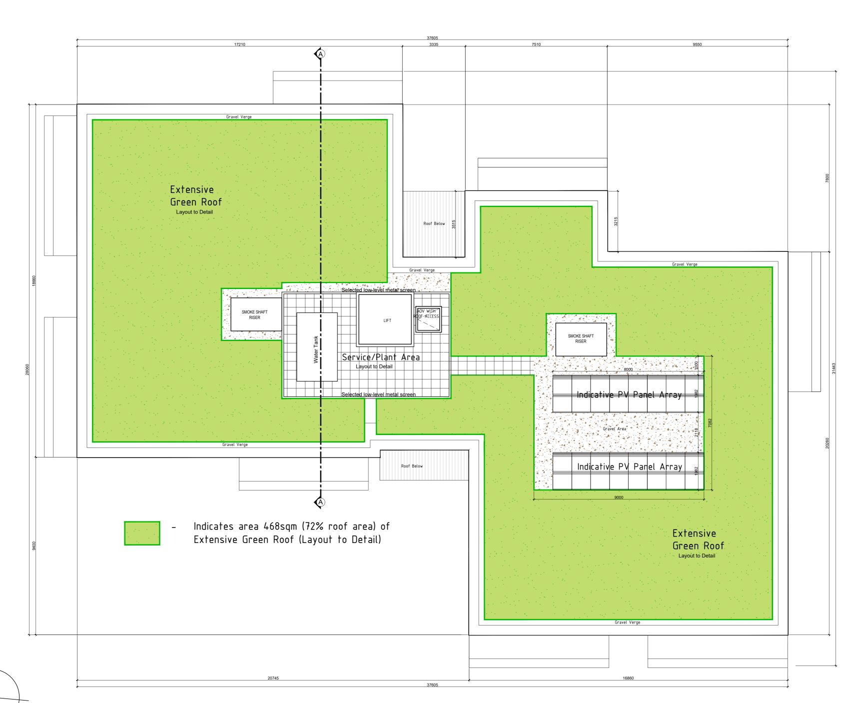
Proposed Block D - Roof Plan Scale 1:100 @ A1
