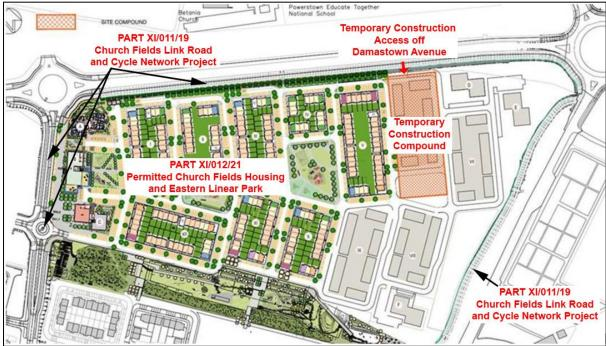
Figure 5.3 Sub-Phase 1A Church Fields East (utilising existing Temporary Site Compound and Access off Damastown Avenue)
