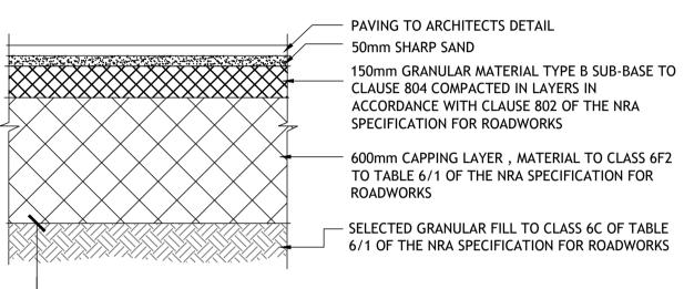
THE CONTRACTOR SHALL CARRY OUT PLATE BEARING TESTS AT 15m GRID ALONG ALL ROADS & CARPARKING BAYS WITHIN THE SITE AT A DEPTH OF 870mm BELOW PROPOSED FINISHED GROUND LEVEL TO ESTABLISH THE CBR%. 450mm x 450mm PLATE BEARING TESTS TO BE CARRIED OUT. THE CONTRACTOR SHALL SUBMIT CBR RESULTS TO ENGINEER FOR REVIEW PRIOR TO PROCUREMENT OF CAPPING LAYER.
