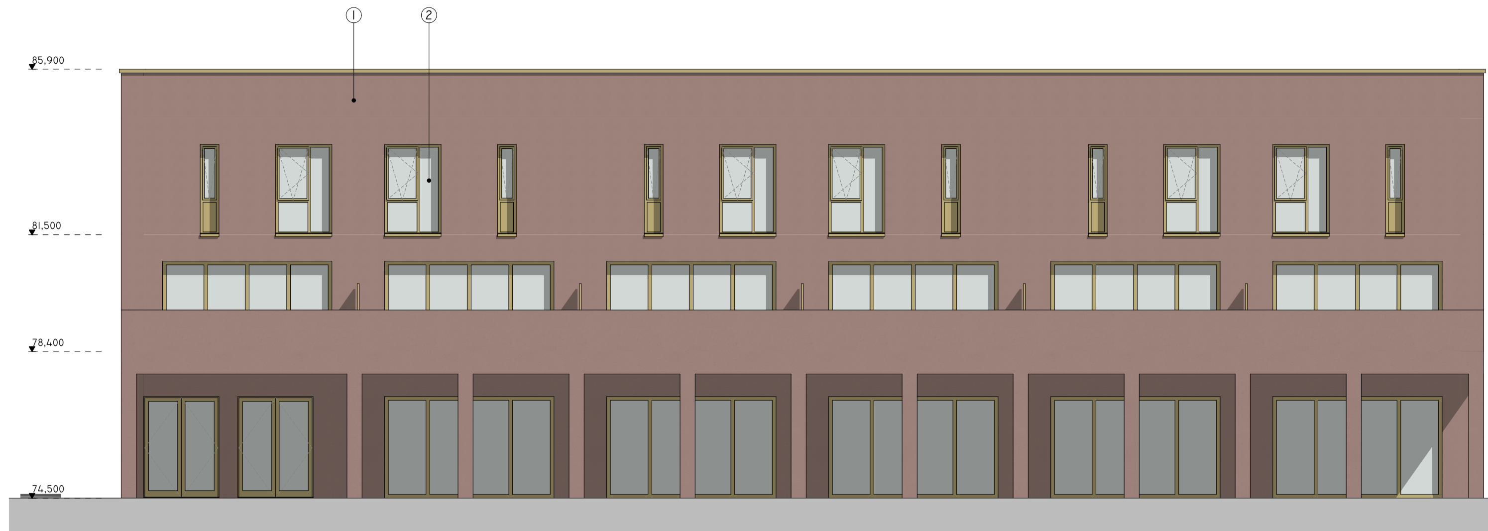
E-C2 BLOCK C SOUTH ELEVATION I-100 P304 1:100
