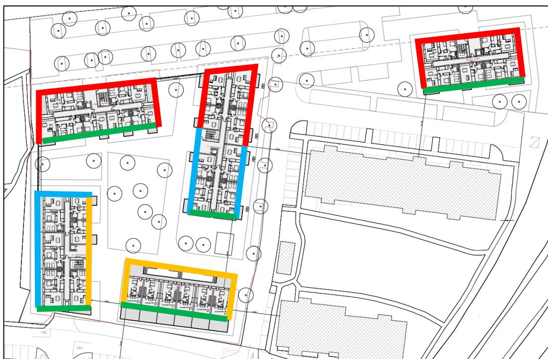
Figure 11 Mark-up of facades that require a minimum sound insulation specification on building elements.
