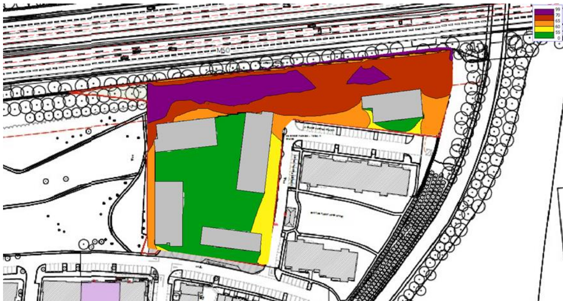
Figure 12 Amenity Noise levels Across the Development Site dB L_{Aeq,16\text{-hour}} at 1.5m height.
