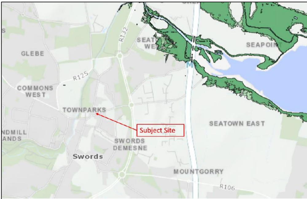
Figure 5-1: Extract from Flood Extents Map: 0.5% (1:200 year) Flood Extent. Source: Site Specific Flood Risk Assessment, Horgan Lynch).
