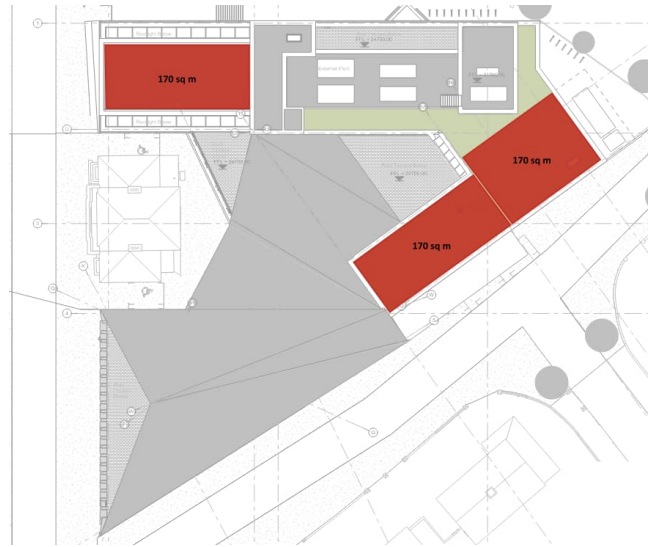
Available roof areas for PV panel installation, highlighted in red
