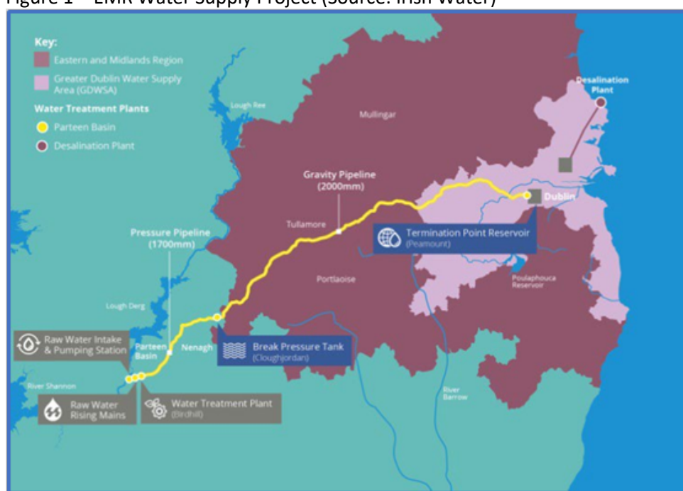
Figure 1 – EMR Water Supply Project (Source: Irish Water)
