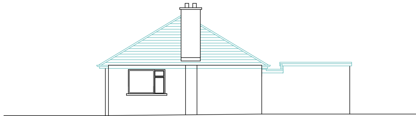
Existing South (Side) Elevation 1:100
