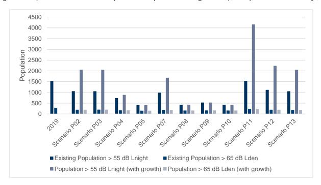
Figure 7.14: Population exposed to levels above the NAO priorities under different runway use and restriction scenarios with and without potential population growth
