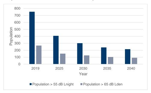
Figure 7.8: Population exposure to aircraft noise levels above 65 dB L<sub>den</sub> and 55 dB L<sub>night</sub> in 2025, 2030, 2035 and 2040 without new measures compared to 2019. Forecast for 2025 – 2040 include population growth.
