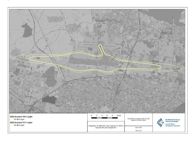
Figure 7.9: 2025 Scenario P01 and Scenario P11 55 dB Lnight exposure contours
