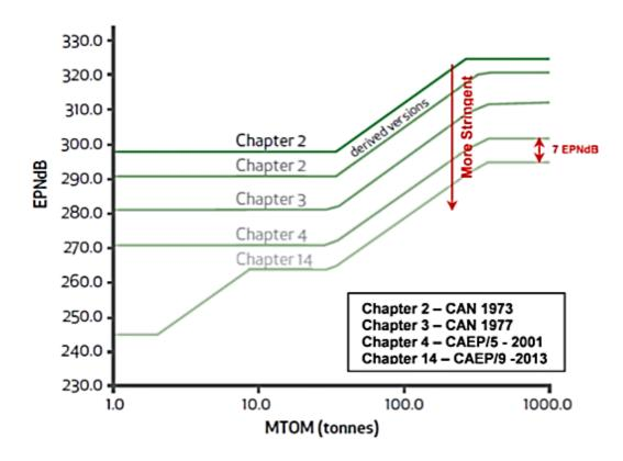
Figure 5.2: Progression of ICAO noise standards. The graphic represents the 'Effective Perceived Noise in decibels' against the Maximum Take Off Mass of an Aeroplane. It demonstrates the improvements in noise limits as ICAO standards have evolved.
