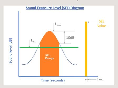
For aircraft overflights, the SEL is always higher than the  $L_{Amax}$ . It is usually the case that the numerical difference between SEL and  $L_{Amax}$  is around 10 dB for aircraft on departure, and 8 dB for aircraft on arrival.
