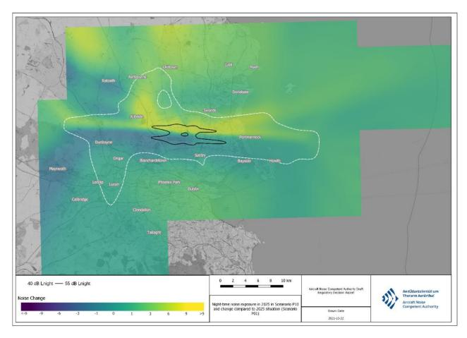
Figure 7.11 55 dB L<sub>night</sub> and 40 dB L<sub>night</sub> in 2025 Scenario P10 with noise exposure changes compared to 2025 Scenario P01 (the noise situation in 2025)
