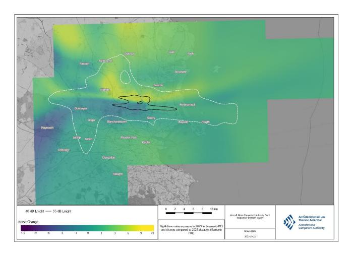
Figure 7.12: 55 dB L<sub>night</sub> and 40 dB L<sub>night</sub> in 2025 Scenario P13 with noise exposure changes compared to 2025 Scenario P01 (the noise situation in 2025)
