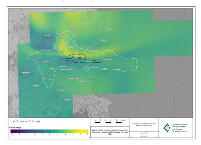
Figure 7.10: 55 dB L<sub>night</sub> and 40 dB L<sub>night</sub> in 2025 Scenario P02 with noise exposure changes compared to 2025 Scenario P01 (the noise situation in 2025)
