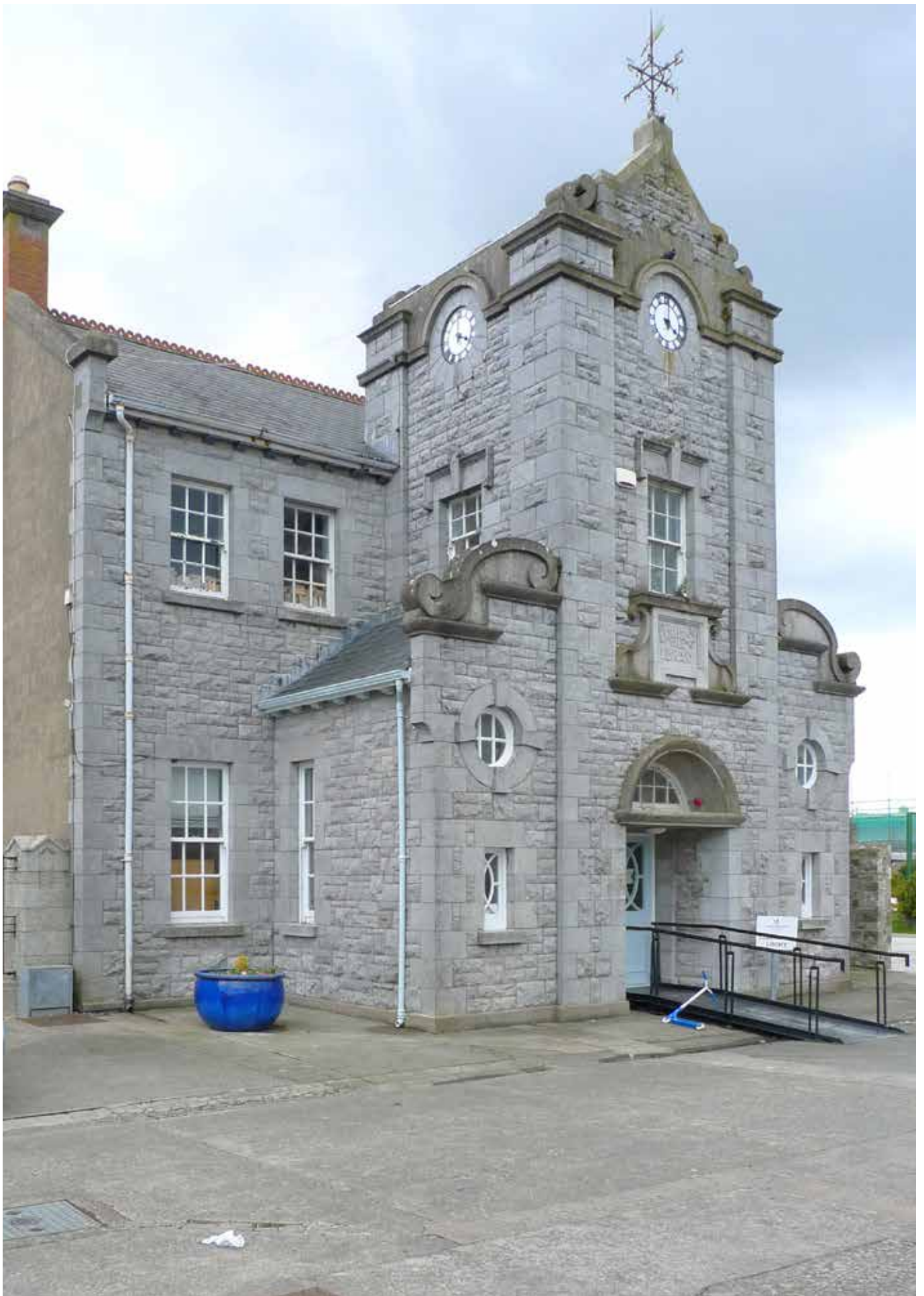
The front facade of Skerries Carnegie Library, facing east onto Strand Street. The facade is finished in coursed limestone, with smooth faced quoins at the corners and around openings, and with the main wall surfaces finished in squared and rough rusticated limestone. Decorative mouldings at parapet level, barge level on the roof, over the entrance door and around the carved plaque bearing the name, all appear to be of a cast composition similar to a fine concrete or artificial stone. The roof is of slate with decorative red fireclay ridge tiles. The two chimney stacks are of red brick.
