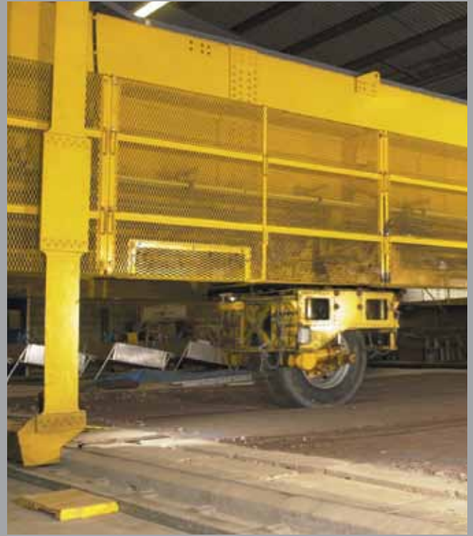
2000 – Full-scale laboratory tests at the UK Transport Research Laboratory comparing Tensar geogrid with alternative forms of geogrid
