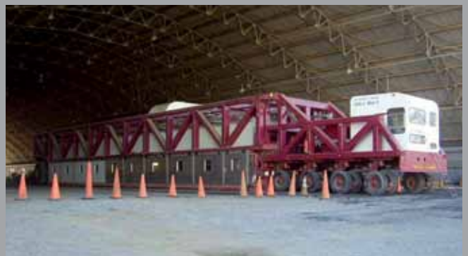
2008/2011 – Controlled environment conditions ensure comparable trafficking test results
